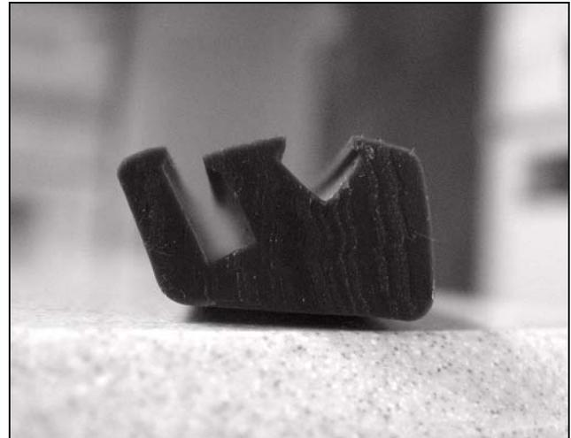
*Here's a cross section of that fixed window seal. Make sure the V-groove is to the outside when you make your cuts and install on your car. Don't fret, this pup will straighten out once your glass and locking strip are in.*
