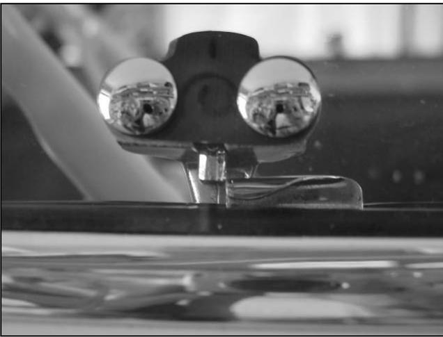
*Here's the sliding window latch in the closed position. You can see the stop slightly descended just above the front side of the latch plate. As Firemarshal Bill suggested, you can double up on that black gasket to push the latch towards the*
