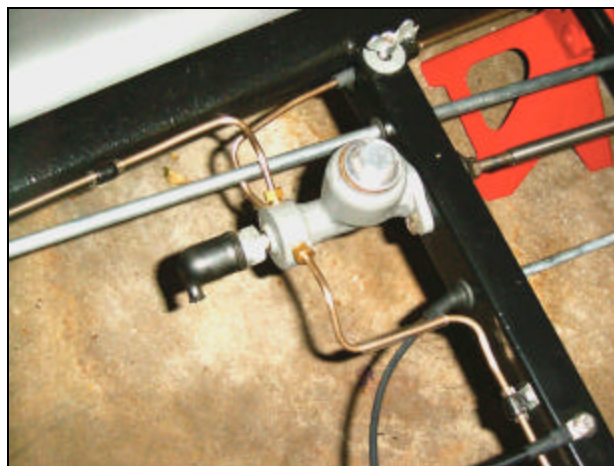
Watch out for the bends in those top two brake lines!
