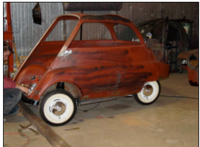
Body of Bubba's one-lung hemi parked back on chassis to check fit of new floor pan.
