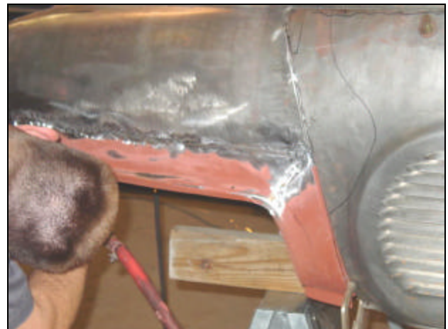
After some expert jockeying, the body shop got Bruce's new panel dialed in. Aaron Bowen of Classic Auto Works puts the finishing touches on the rough-in.
