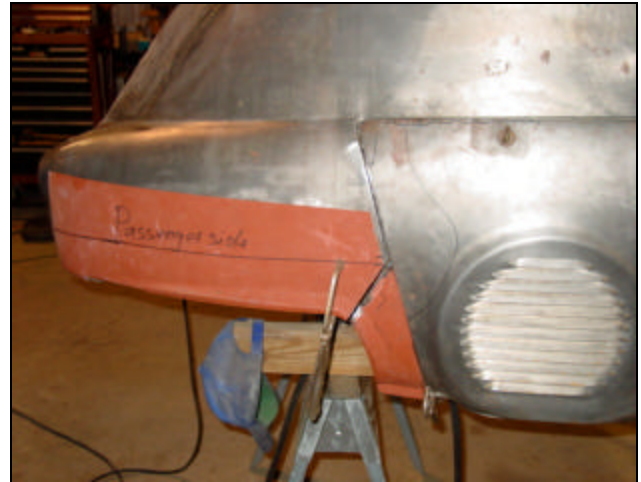
Note diagonal cut that had to be made in repro quarter panel on Bruce's car. These guys aren't stamped from original dies and, while close, this one did not fit correctly as delivered.
