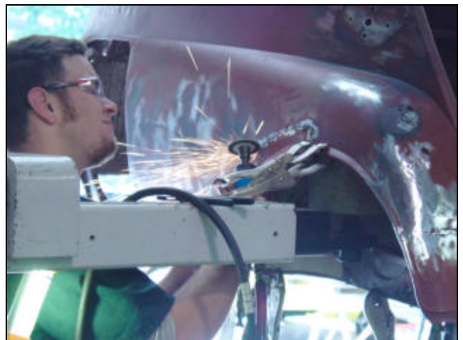
You'd think getting' your bottom flamed would be enough! Robert's car meets Mr. Grinder while the new outer wheel well panel gets fined tuned. It's getting' there!
