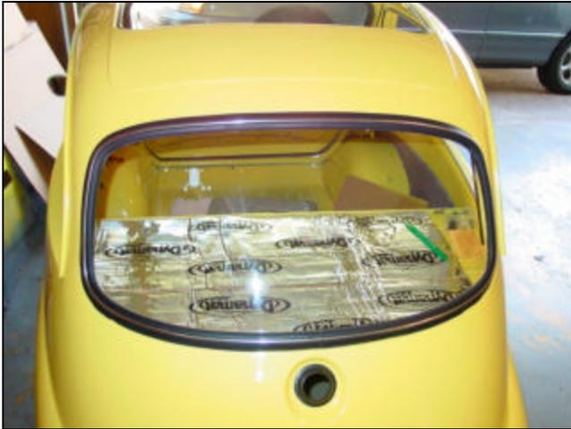
*Dynamat Extreme acoustic and heat insulation on rear deck of Bruce's car. New window seal, lock strip and external rubber seals have just been installed too.*
