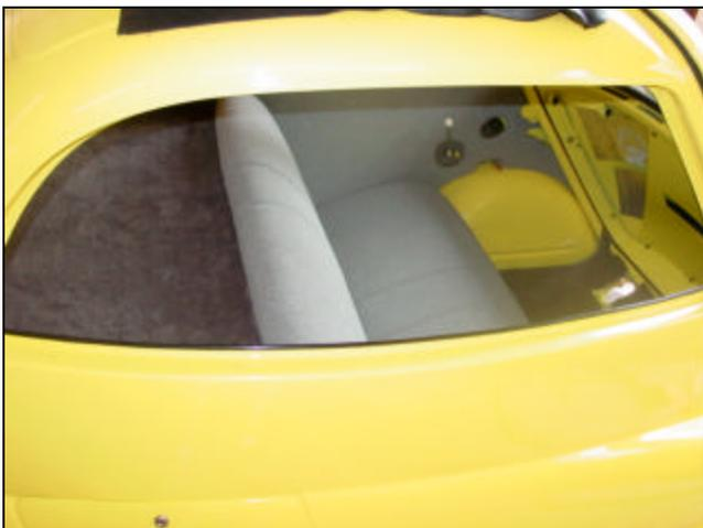
Brand new seat, side panels and carpet in Bruce's car. Door panel is next. The door panel was easily the biggest time consumer in terms of labor to reconstruct a new one even though the original was used for a template.
