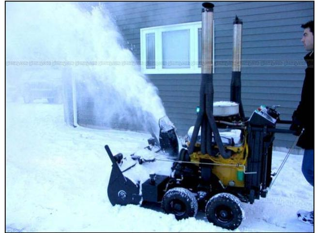
In order to get those two snowed-in Isettas at the top of Page One uncovered, we've enlisted the services of this **V-8 powered snow blower**. This bad boy is based on a **big-block 454 Chevy** motor cranking 412 HP. It'll throw snow 50 feet at 3,500 RPM's. Check out all the action at [www.v8snowblowers.com](http://www.v8snowblowers.com). Also click on the "Gas Blender" link for a sneak preview of the **high-performance blender** they're whippin' up.
