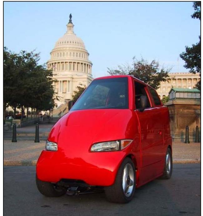
Tango anyone? **Gerron Hite** called our attention to this **Tango T600** on eBay a while back. 0 - 60 mph in 4 seconds using a half ton of battery power. The "car of the future" is slimmer than a Honda Gullwing bike and runs 80 miles on a charge, recharging to 80% capacity in 10 minutes. Hmm ..
