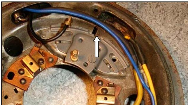
*Here you can see the small oblong notch in the Dynastart housing just above the points bracket. The center V-notch sits just to the right of it at the bottom.*
